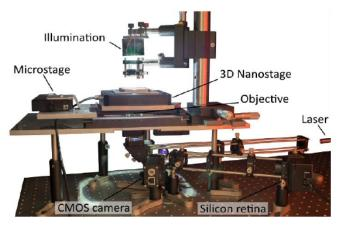
The system exhibits very good performances regarding the resolution while measuring forces. We have demonstrated that a resolution of 10pN can be reached. However, these performances have been obtained while degrading the ease-of-use. This is not only due to the mechanical structure of the platform but also to the complex command laws.
