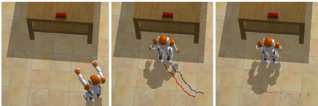
**Figure:** The approach task modeled in Webots. On the left, the robot's original pose. In the center, the followed path. On the right, the desired pose with respect to the red can on the table
