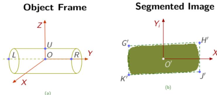
**Figure:** Definition of the cylindrical container object model. a) 3D representation of the object frame  $O$  and the definition of four points of interest. b) Segmented blob and image features defined from the oriented bounding box.
