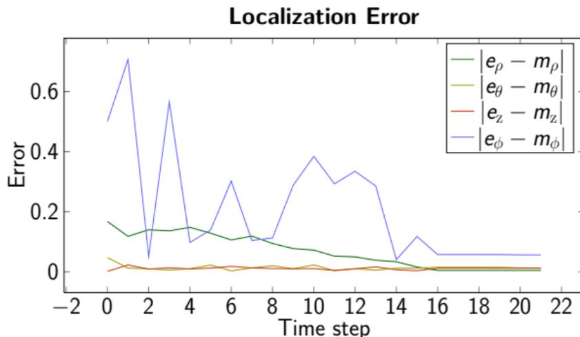
**Figure:** Evolution of the localization error between estimations  $e$  and measurements  $m$ .
