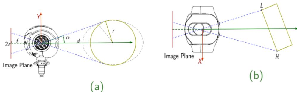
**Figure:** Estimation of the object's depth. a) The model assumes  ${}^C O_\theta = 0$  in (9), b) XZ visualization of the scenario where the circumference corresponds to an ellipse and the distance from the projective ray and the center  $O$  is larger than  $r$ .
