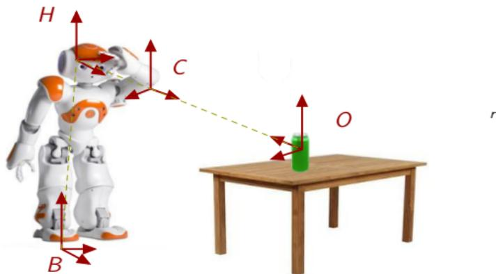
**Figure:** Definition of the reference frames to solve the localization task. In the image,  $B$  corresponds to the base frame,  $H$  to the head frame,  $C$  to the camera frame, and  $O$  to the object frame.
