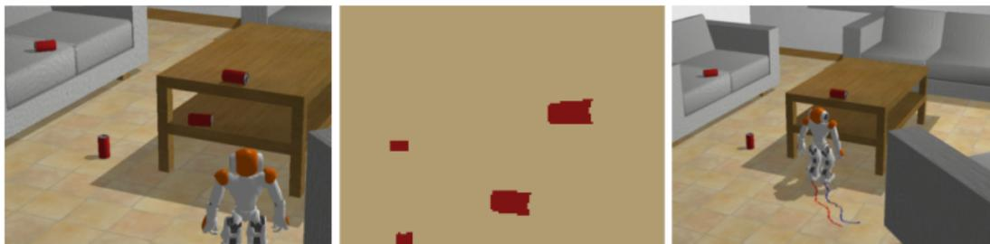
**Figure:** Top-down feature attention testing. On the left, the robot's original pose. In the center, the on-board view of the frame on the left. On the right, the trajectory followed. Despite the number of red cans, the agent was able to track the one on the top of the table.
